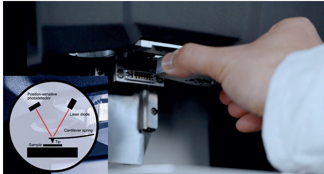
Fig. 1. Insertion of the actuator body with cantilever into the AFM: the z-sensor is integrated in the compact and lightweight actuator body without any cables © Anton Paar
